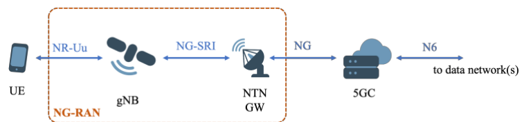
Figure 5. NTN architecture with regenerative payload and direct access, full gNB on-board.
